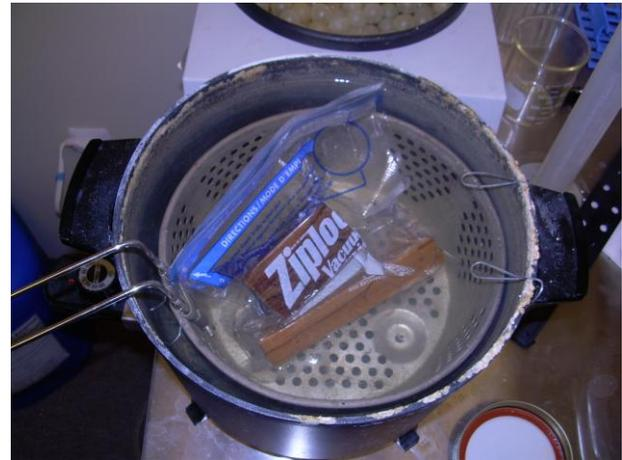
Upon completion of curing, permit the wood to air-cool to room temperature. Trying to cool the wood rapidly will adversely affect the hardness of the cured stabilizer.
