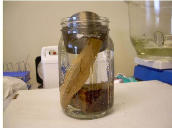
Apply the maximum vacuum to the chamber that your system will permit. The length of time required at vacuum will vary depending on the system and the type/size of wood and will require some experimentation. A high vacuum (<10 mBar) high flow system (>27 cfm) running continuously can fully evacuate spalted pen blanks in about 20 minutes. Other systems may require hours or even days at vacuum.
