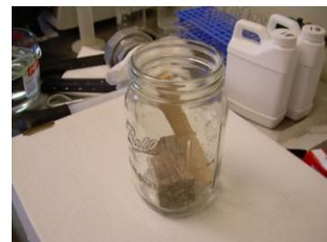
Place your wood pieces in a container and weight them down to prevent floating. The container should be tall enough to prevent foaming over the sides during stabilization.
